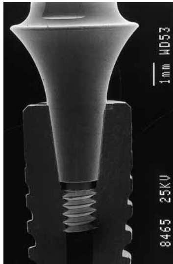
Fig. 1 The internal fastening screw allows free positioning in rotational symmetry for the Ankylos abutment. The conical connection turns the two-part implant into a virtual one-part implant.
